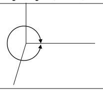
Angles about a point add up to  $360^{\circ}$  or 4 right angles  $(4 \times 90^{\circ})$
